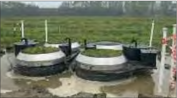
Lysimeter stations after the installation of the waterproof collars and deinstallation of the groundwater lowering
