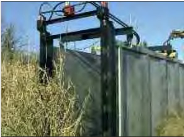
Fen lysimeter vessel with monolith cutting tools
