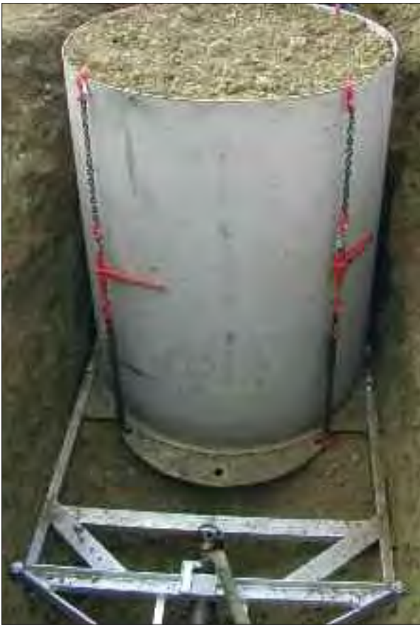
Base cutting with a steel plate of a 2 m² soil monolith
