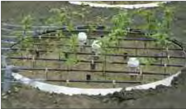
Lysimeter with irrigation system and young beeches
