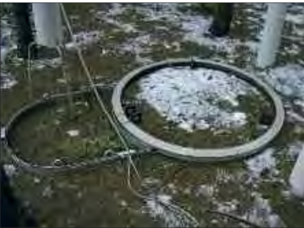
High grade steel lysimeter with planted hatch
