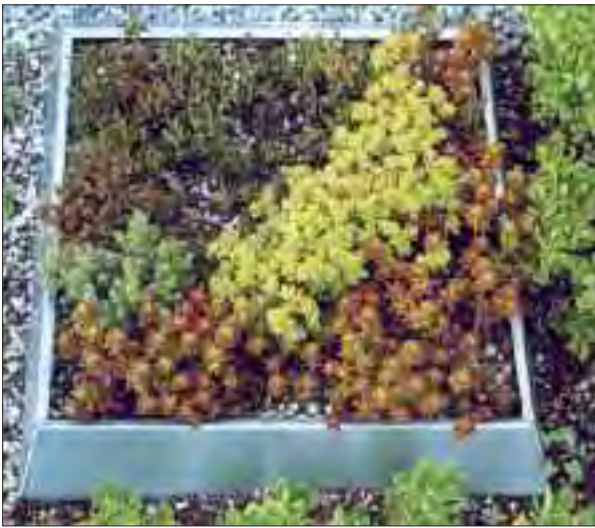
Green roof lysimeter
