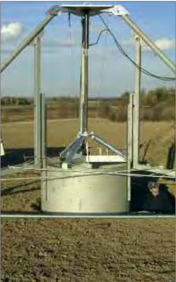
Excavation Technology for a 2 m 2 soil monolith
