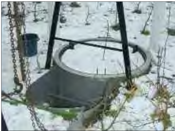
High grade steel lysimeter in winter
