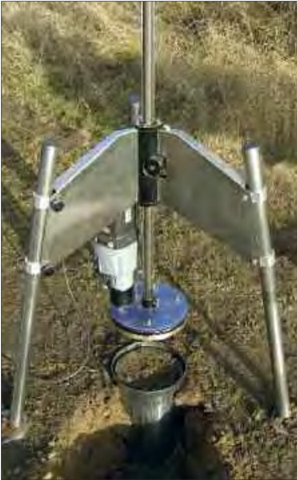
Cutting of a 0,03 m 2 (Ø 20 cm) laboratory soil column
