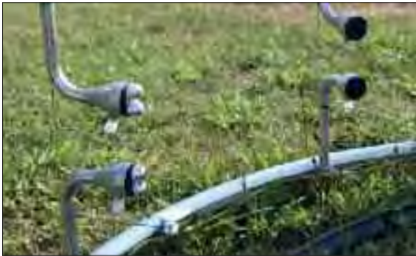
Ultrasoundsensors and intake port for the gas analyzer
