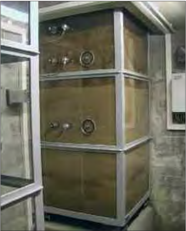
Weighable lysimeter with soil hydraulic sensors
