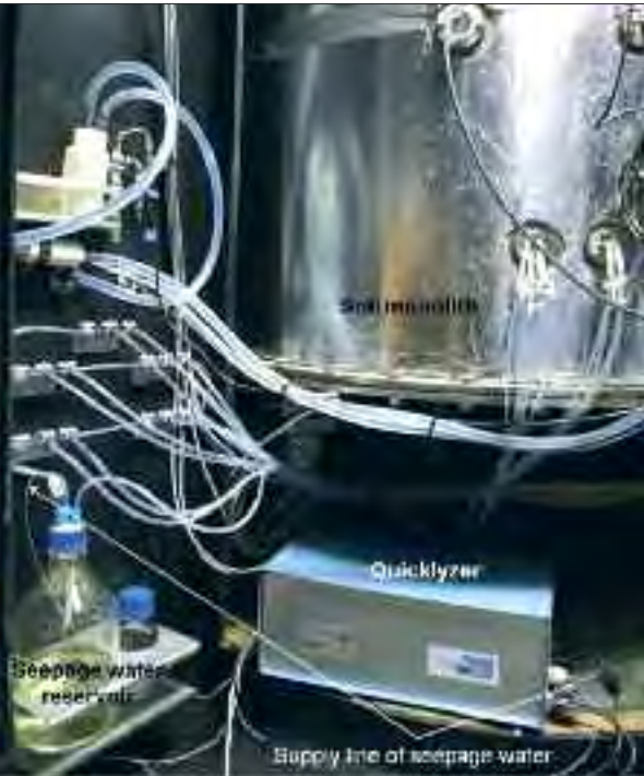
Quicklyzer installed at a lysimeter
