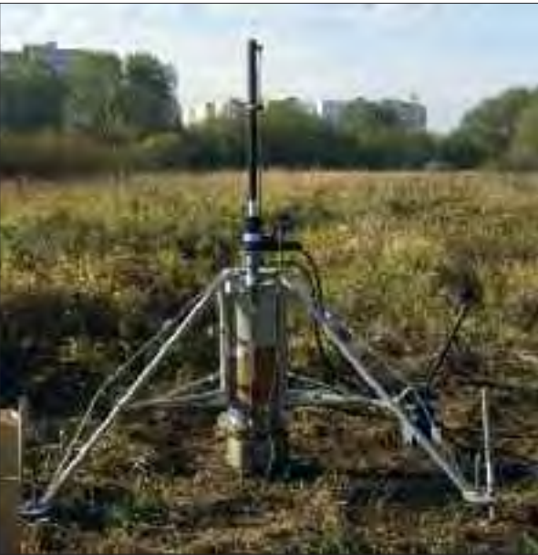
Cutting technology for laboratory soil columns in plastic vessels in use at the Oka floodplain
