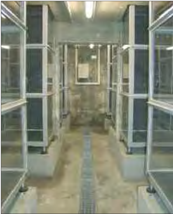
Root Stack with 8 lysimeters
