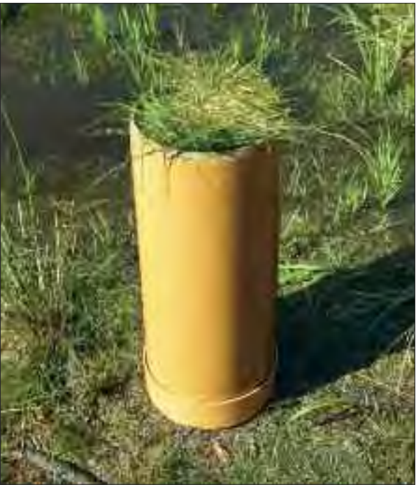
Fen soil column with a diameter of 200 mm
