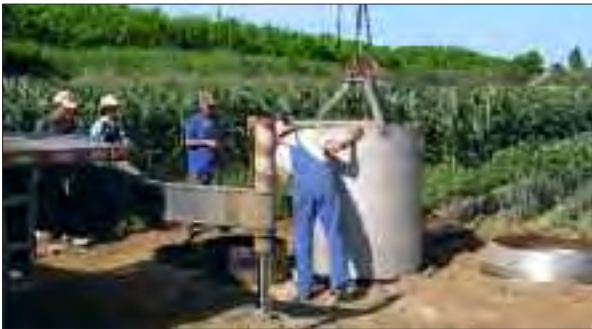
Freshly excavated soil monolith in a stainless steel vessel
