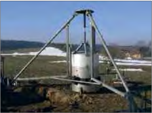
Excavation Technology for a 1 m 2 soil monolith
