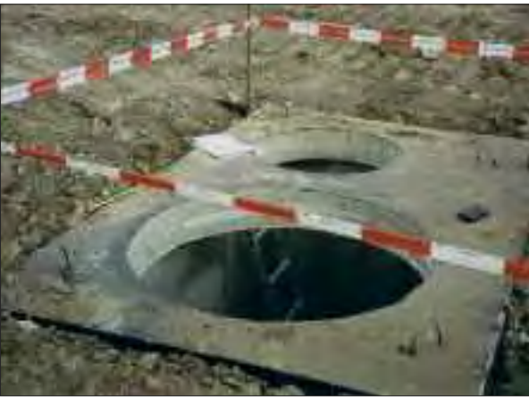
Top panel of a containerized concrete lysimeter
